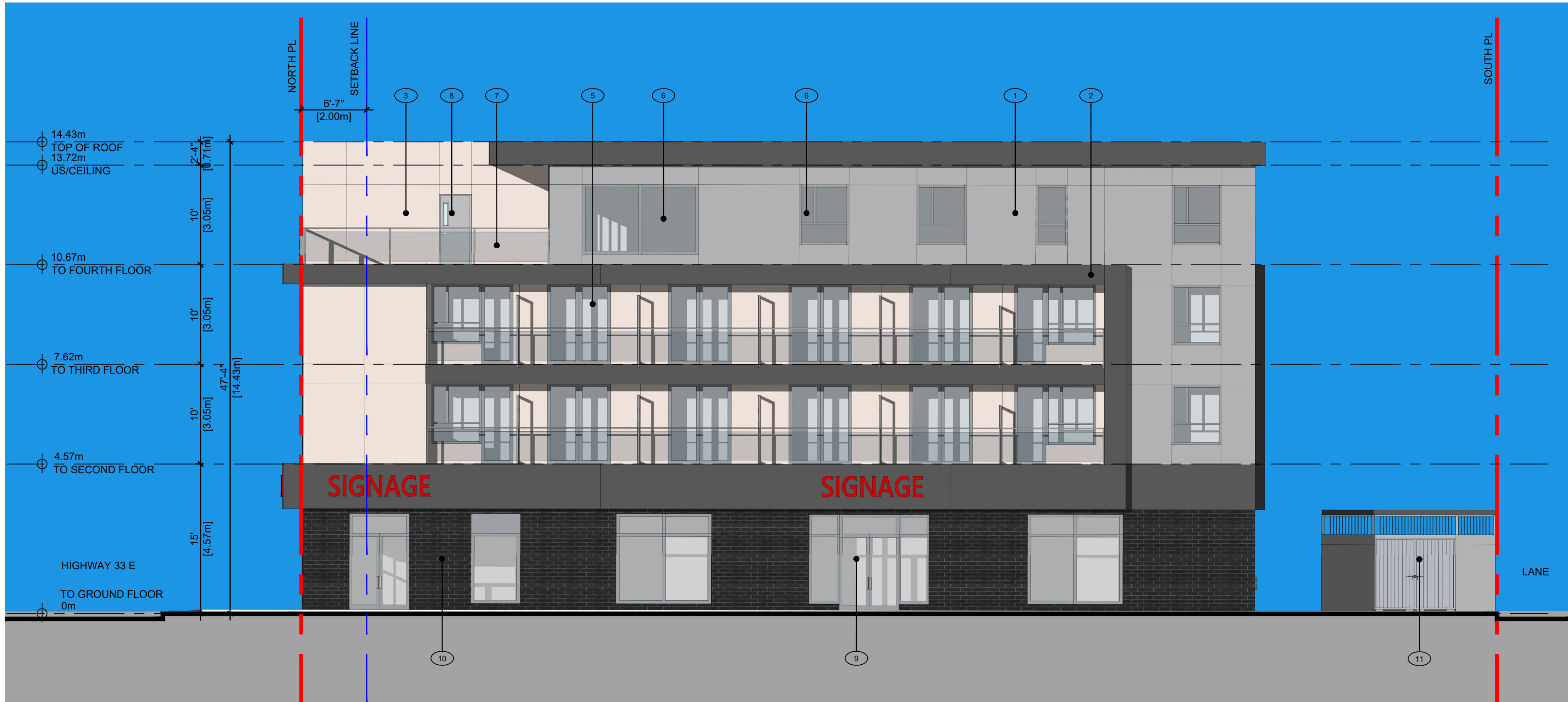
3 BUILDING ELEVATION-WEST Scale: 1/8"= 1'-0"
